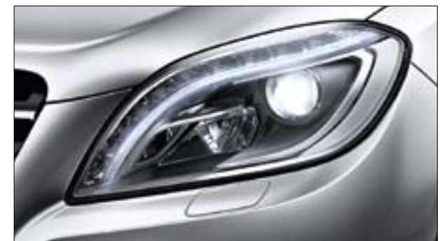
Adaptive High Beam Assist automatically maximises the range of the headlamps, thereby improving visibility for the driver
