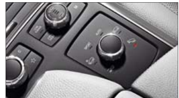
The desired mode is selected via a rotary switch in the centre console
