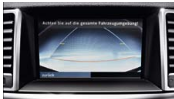
The reversing camera uses the central display to allow you to see what's immediately behind the car
