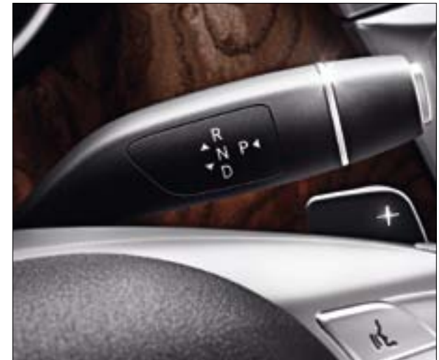
Transmission operation with the Direct Select lever – the driver can also control gear shift operation via the gear shift paddles on the steering wheel
