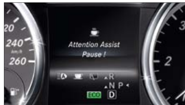
If it detects signs of fatigue or concentration lapses, Attention Assist suggests taking a break
