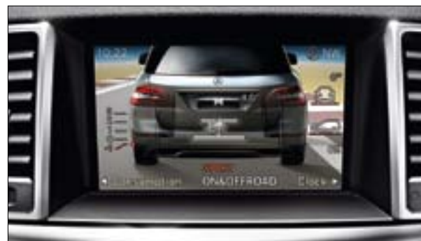
The COMAND Online display shows the current driving mode along with the gradient and angle of inclination
