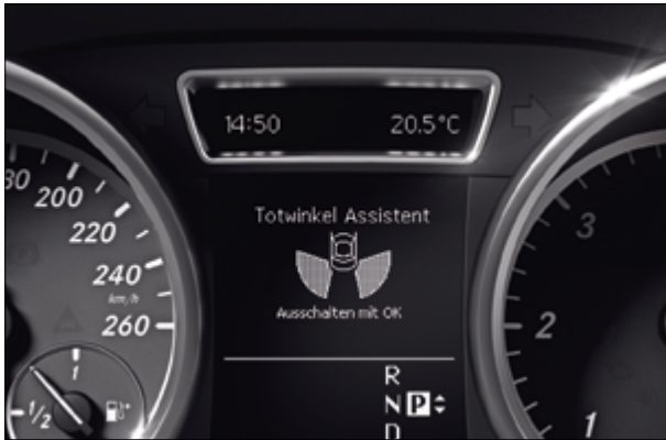
Active Blind Spot Assist increases safety during lane changes
