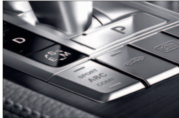
The Adaptive Damping System ADS can be individually adjusted at the touch of a button
