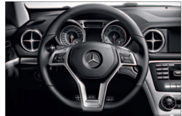
The multi-function steering wheel with nappa leather and gear shift paddles
