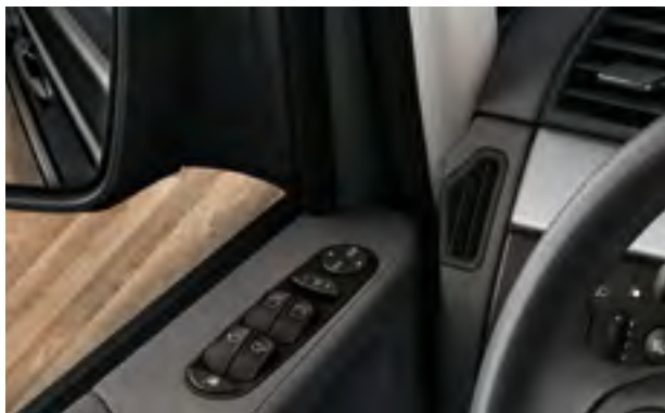
Control unit for electric front windows, vent windows and door mirrors
