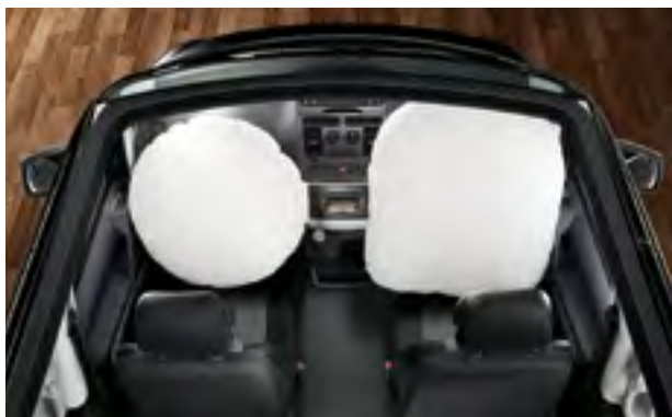
Driver and front passenger airbags (activated, at maximum deployment)
