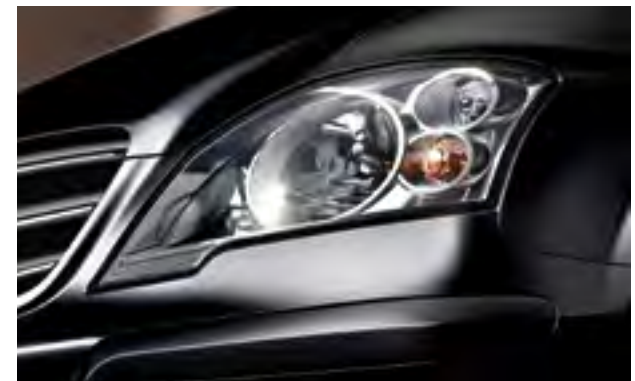
Bi-xenon headlamps with LED daytime running lights and halogen fog lamps
