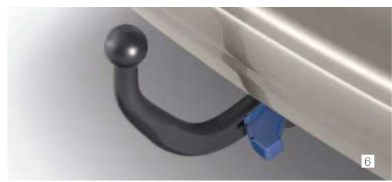
6 De-mountable swan neck tow bar For those customers wanting a neater installation. The lockable swan neck tow ball assembly of this tow bar can be quickly removed when not in use.
