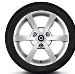
6-spoke alloy wheels 38.1 cm (15"), design 3 , set, for front tyres: 175/55 R15; rear tyres: 195/50 R15.
