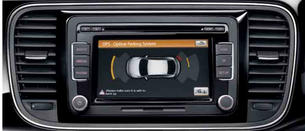
Parking sensors , both front and rear, assist in parking manoeuvres by emitting both audible and visual warnings, alerting the driver to any obstacles: the closer you are to an obstacle the faster the sound frequency. In addition an optical parking display extends the functions of the parking sensors by indicating your position during parking on the touch-screen colour display of the RCD 510 DAB radio. Not only do they make it easier to park, but safer too, as you are more aware of any obstacles that may be in your way.
