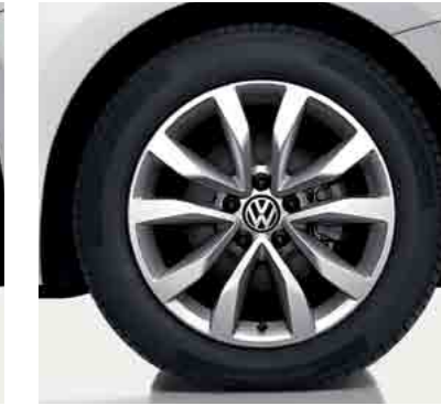
17 inch 'Rotor' alloy wheels with 215/55 R17 tyres and anti-theft wheel bolts. No cost option on Design.
