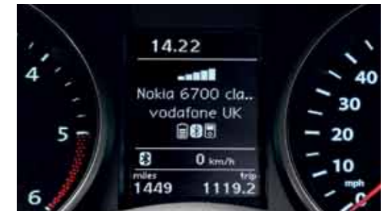
Bluetooth telephone connection for HFP (Hands Free Profile) enabled telephones allows you to use your mobile phone safely and easily. Call information is displayed on the multifunction computer (Highline) which now also displays a Bluetooth symbol to inform you of your phone's continuous pairing with the vehicle.
