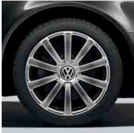
'Omany' 9J x 19 inch alloy wheels* with 255/40 R19 tyres and anti-theft wheel bolts. Optional on all models.
