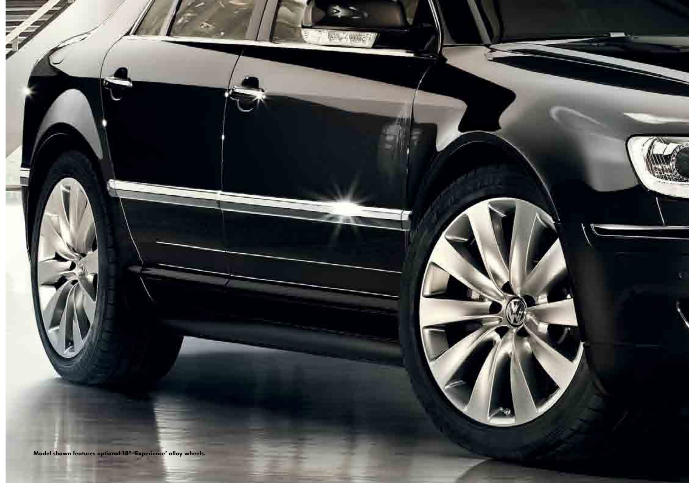
'Omany' 9J x 19 inch alloy wheels* with 255/40 R19 tyres and anti-theft wheel bolts. Optional on all models.
