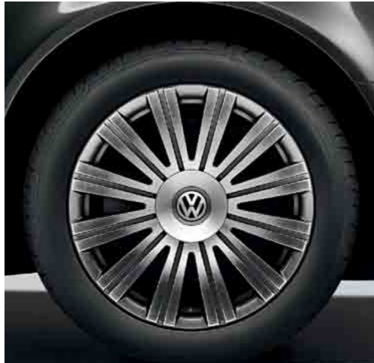
'Performance' 8½J x 18 inch alloy wheels with 255/45 R18 tyres and anti-theft wheel bolts. Optional on all models.
