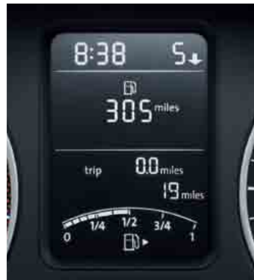
The multifunction computer (Midline) displays current fuel consumption figures on the display screen, and also makes recommendations for optimal gear changes on the 1.4 litre 85 PS and diesel models.
