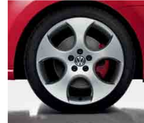
'Monza' 7 1/2 J x 17 alloy wheels with 215/40 R17 tyres and anti-theft wheel bolts give the GTI a sporty intent, while the red brake calipers help to create an even more stylish exterior. Standard on GTI models.
