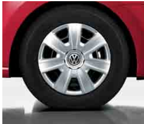
14 inch steel wheels with 175/70 R14 tyres and full size wheel trims feature a robust seven spoke design, adding a sporty touch. Standard on S models.
