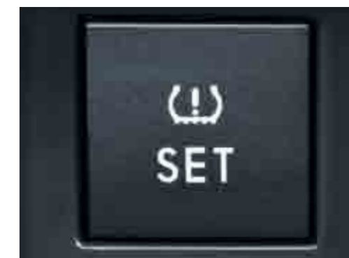
In the event of a change in tyre pressure, the tyre pressure indicator alerts the driver via a warning in the multifunction display. Not only does correct tyre pressure ensure a high degree of safety, but it also helps extend the life of the tyres and reduces fuel consumption.
