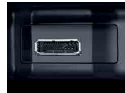
The MDI (Multi Device Interface) connects you to external audio sources, such as USB or iPod, which you can operate via the radio or optional navigation/radio system.
