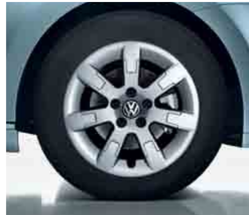
'Greenland' 5 1/2 J x 15 light alloy wheels with 185/60 R15 low rolling resistance tyres help to reduce the BlueMotion's fuel consumption. Standard on BlueMotion models.
