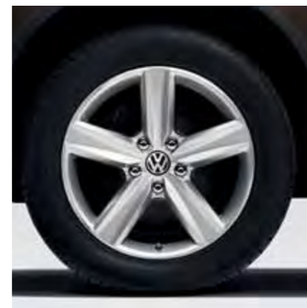
'Girona' 9J x 19 inch alloy wheels with 265/50 R19 tyres add a touch of real style. Optional on Escape models. No cost option on SE and Hybrid models.
