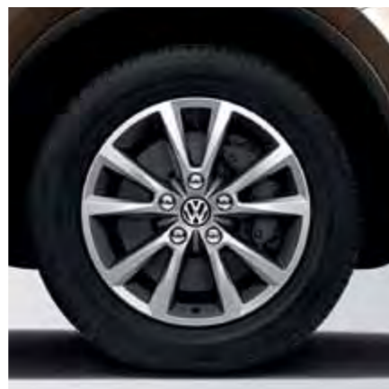
'Karakum' 8J x 18 inch alloys, with 255/55 R18 tyres are eye-catching and bold. Standard on Escape models.
