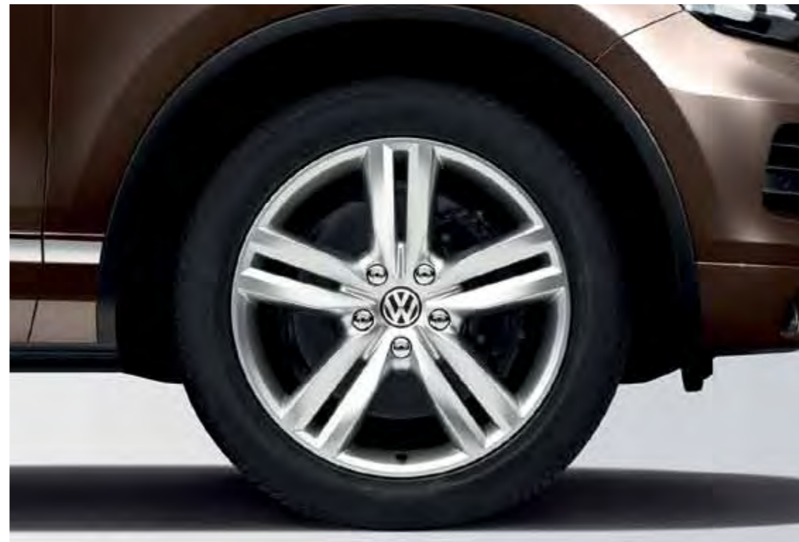
'Pikes Peak' 9J x 20 inch alloys, with 275/45 R20 tyres deliver real individuality. Standard on Altitude, optional on SE, Escape and Altitude V8 models.
