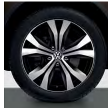
'Tarragona' 9J x 20 inch alloys, with 275/45 R20 tyres and anti-theft wheel bolts create an exclusive look. Standard on Altitude V8 models, optional on SE, Escape and Altitude models.
