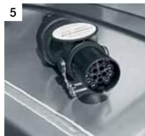
**Trailer socket, 24 V.** For a safe electrical connection between tractor and semitrailer or trailer. The socket can be used to power headlamps, tail lights, brake lights etc.
