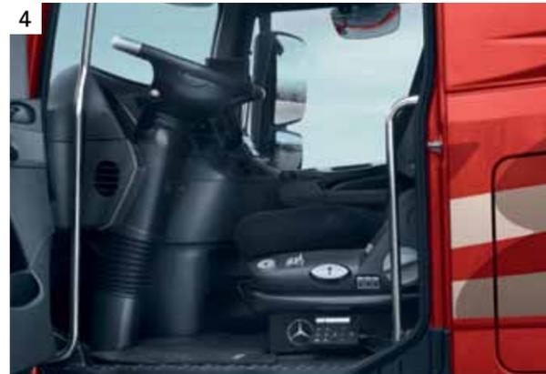
**5 3 Backlit Mercedes-Benz star logo.** Shining detail: at the touch of a button the white-backlit Mercedes-Benz star logo (Code FA6) provides even more lustre. LED lighting with output of 1.9 W and diffuser lens. Installation kit for retrofitting consists of: star logo, incl. LED, switch, wiring harness and mounting materials.
