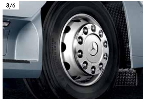
**Stainless steel wheel trim and wheel nut cap set.** Because every detail counts: the wheel trim and wheel nut cap set protects the wheel and the wheel nuts from damage and adds highlights to your Actros or Antos. For 57.15 cm (22.5") wheels.
