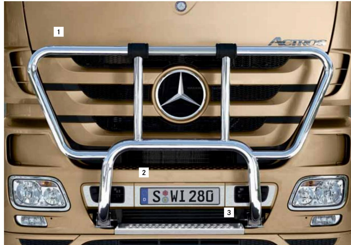
**Front bar.** An effortlessly superior look: the robust front bar emphasises the Actros's distinctive appearance. A perfect fit for vehicles with underguard. Supplied with mounting support. Material: tough, hand-polished stainless steel.
