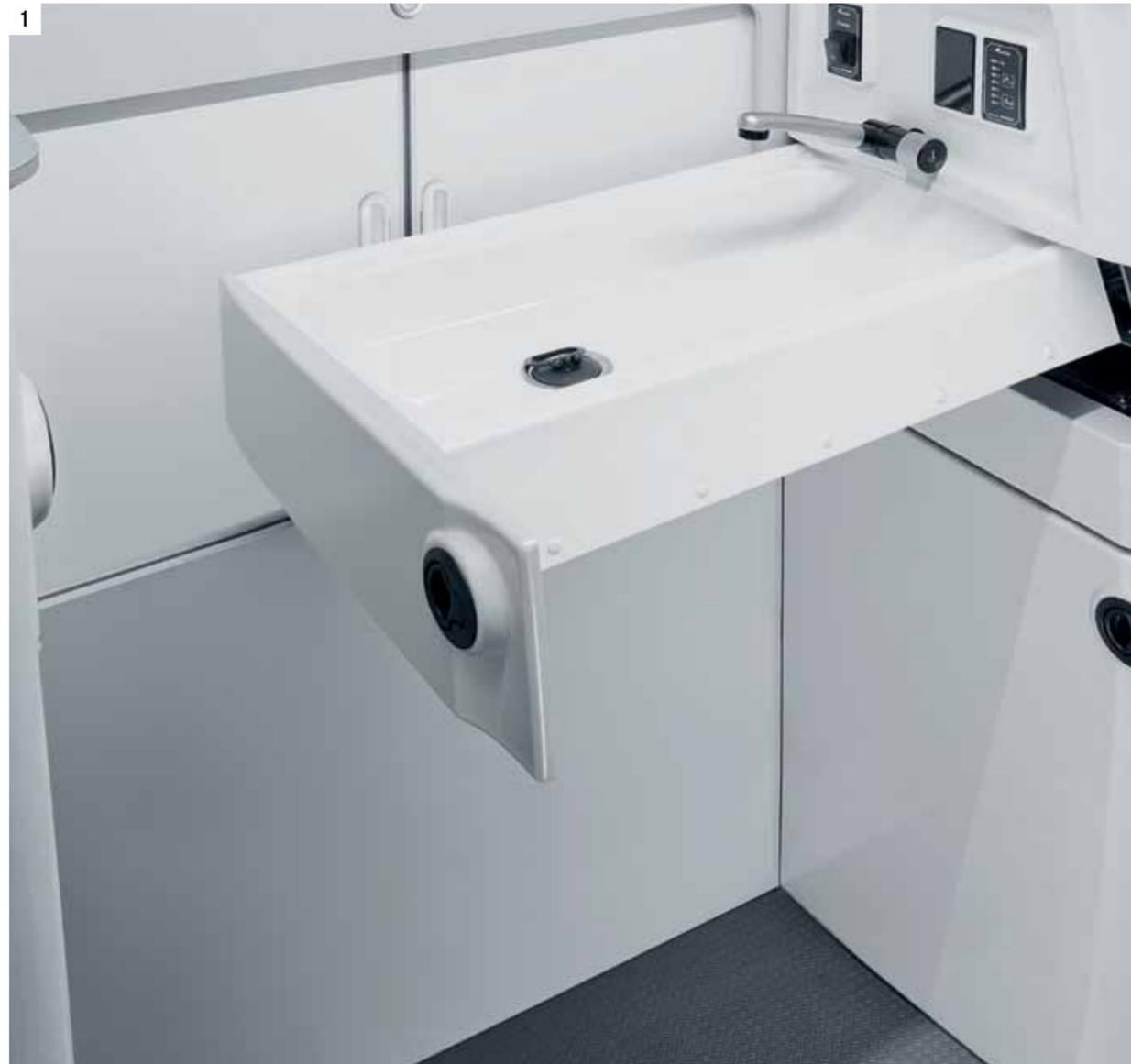
**1** **2****3** The tower behind the driver's seat features a pull-out washbasin. A hose pump is used to fill up with 20 litres of fresh water from outside.
