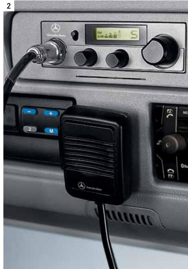
**1 1 2 3 Ac An Universal CB radio, 12 V.** At home on all channels: universal CB radio with 3 switchable national frequency tables: 80 FM channels, 4 W/12 AM channels, 1 W/40 FM channels, 4 W/40 AM channels, 1 W/40 FM channels, 4 W/CEPT. With ASC (automatic sound control) and microphone with up/down buttons for selecting channel. B6 683 0017
