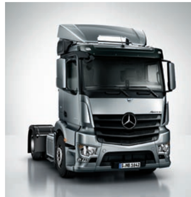
The ClassicSpace M-cab 1) is available with a 170 mm or 320 mm 2) high engine tunnel. With its length of 2000 mm, it presents an optimum solution for virtually any application. Also available is the CompactSpace M-cab 1) , whose flat roof makes it ideal for over-cab bodies.
