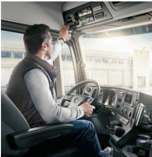
FleetBoard Time Management: after the driver card has been inserted into the FleetBoard on-board computer, all the data are downloaded from the driver card to the haulage company at the touch of a button. This saves time and administration while meeting all legal requirements.
