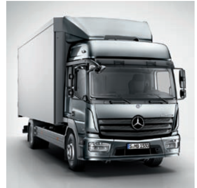
L cab BigSpace. With a high roof and measuring 2295 mm in width and 2250 mm in length, the L cab BigSpace offers great freedom of movement and plenty of stowage space. It is ideal for operations involving frequent overnight stays on board
