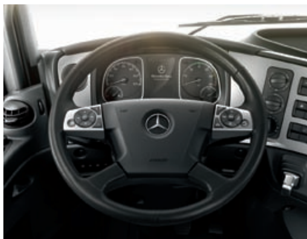
Multifunction steering wheel. The standard-fit multifunction steering wheel makes light work of various functions: apart from the radio and telephone, the cruise control can now also be operated via the steering wheel. Many other vehicle functions and diverse settings can also be controlled in the new instrument cluster
