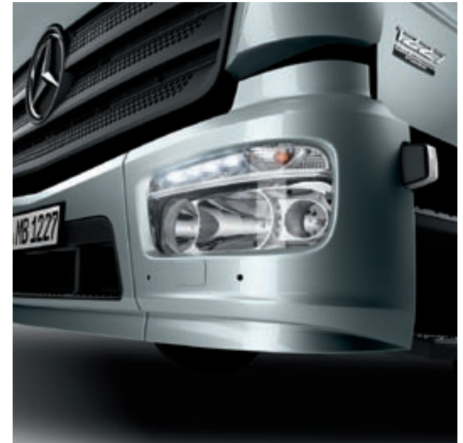
LED technology. Apart from highlighting the Atego’s distinctive design, the optionally available LED daytime running lamps also cut costs, as the LEDs are designed to last throughout the Atego’s useful life. LED side marker lamps and tail lamps are optionally available
