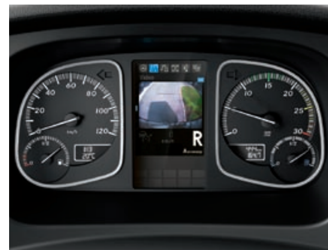
12.7 cm TFT colour display. The new Atego is optionally available with an instrument cluster incorporating a 12.7 cm TFT colour display and video function. The images from an optionally 1) available reversing camera can be viewed on this display, for enhanced safety during manoeuvring, for example
