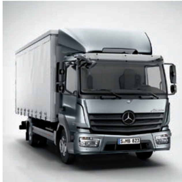
S cab ClassicSpace. Measuring 2295 mm in width and 1650 mm in length, the S cab ClassicSpace combines a comfortable workplace with a high level of visibility and full body length. Just the set-up to tackle narrow alleys and backyards with ease
