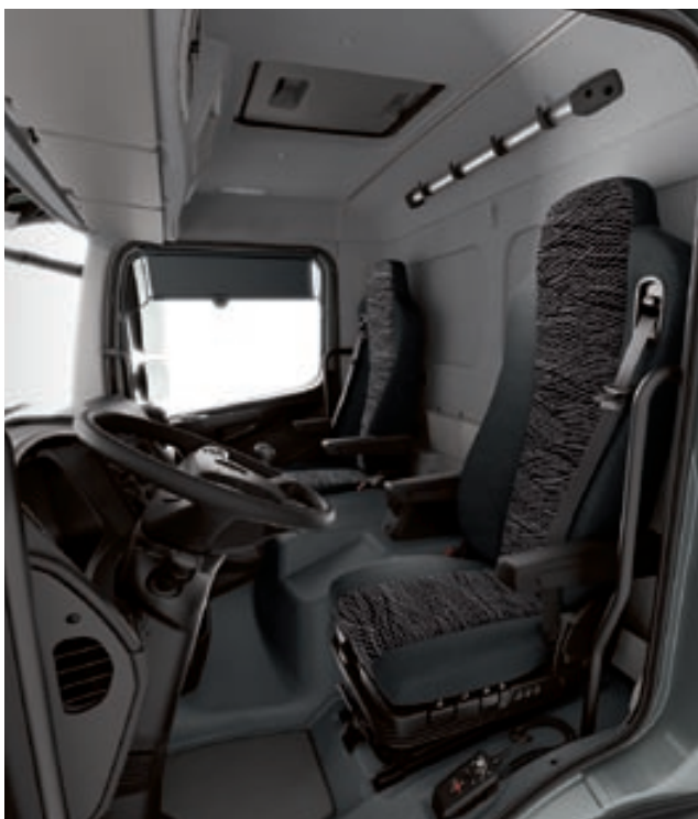
High seating comfort. The comfort suspension seat is optionally available for the driver's and co-driver's side, boasting folding armrests 2) and integrated belt height adjustment along with a host of other comfort features
