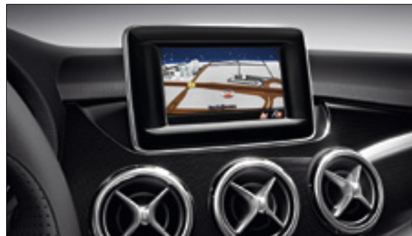
The Becker® Map Pilot navigation system shows vital information both via the Audio 20 radio/single CD display, and the multi-function colour display
