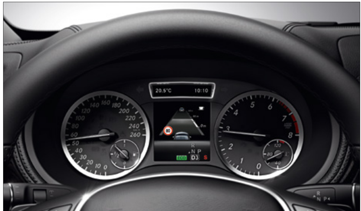
The Speed Limit Assist alerts the driver to the current speed limit
