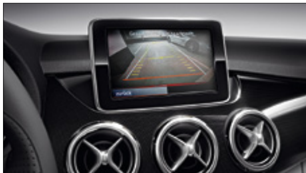
The central display shows the area behind the car during a parking manoeuvre
