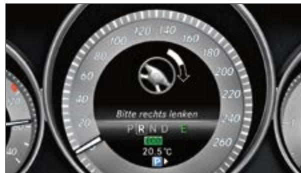
At speeds of up to 20 mph, Parking Guidance can automatically measure the length of parallel parking spaces
