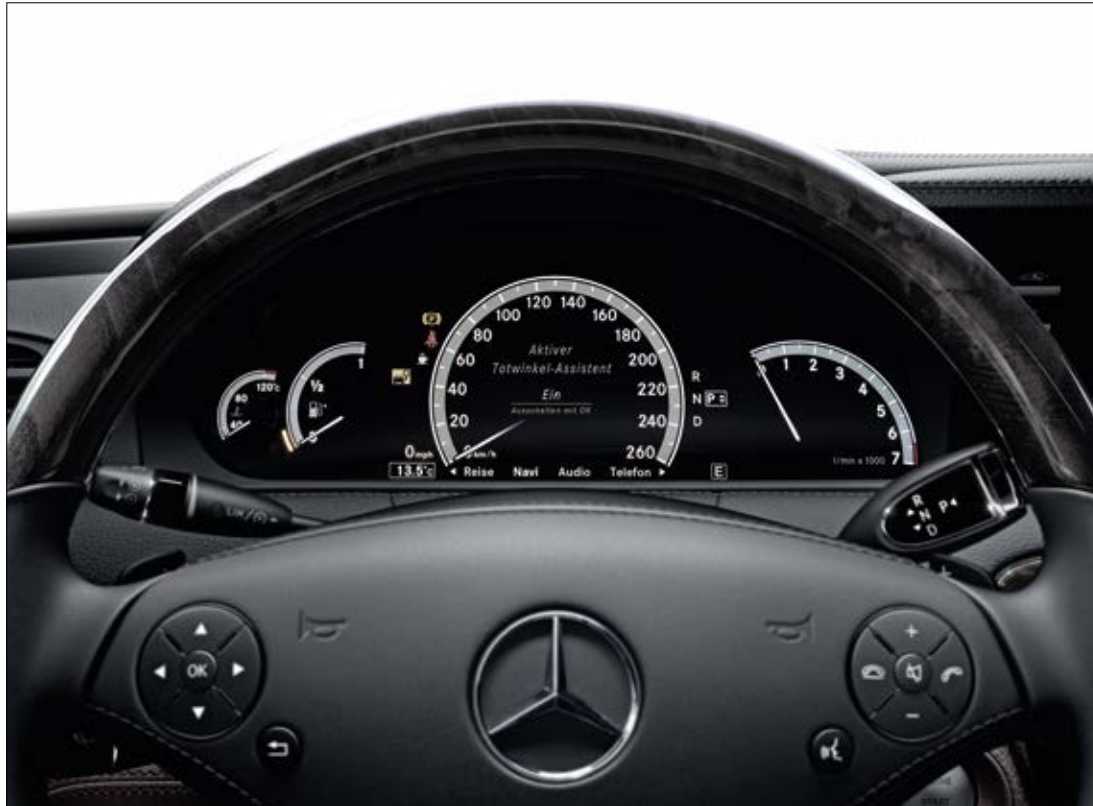
The Driving Assistance Package combines Active Blind Spot Assist, Distronic Plus and Active Lane-Keeping Assist
