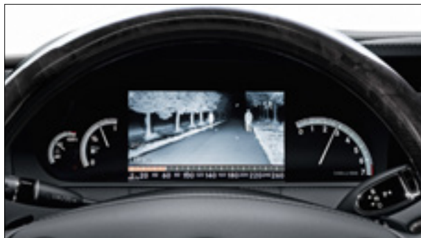
Night View Assist Plus helps drivers to spot pedestrians by highlighting them on the screen
