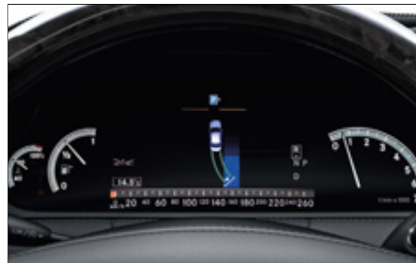
The progress of the manoeuvre is shown in the multi-function display
