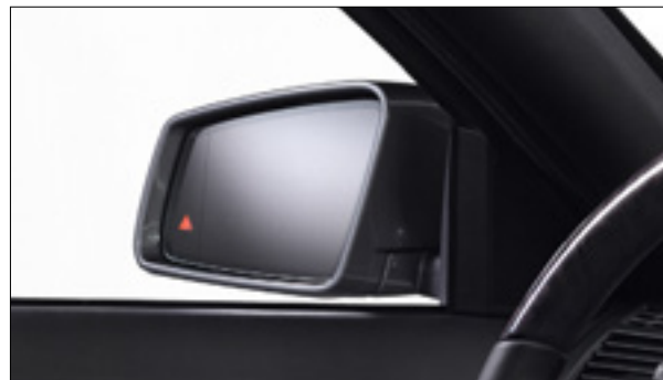
Active Blind Spot Assist warns the driver of potentially dangerous lane changes
