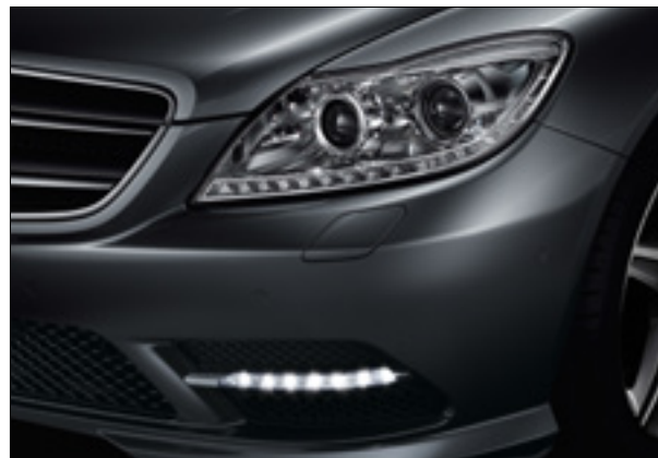
Intelligent Light System with bi-xenon headlamps and LED daytime running lights
