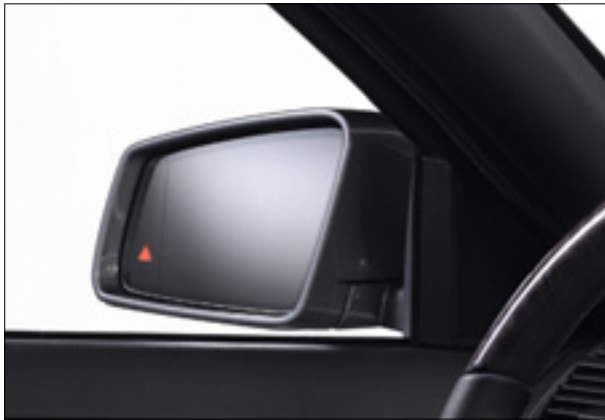
Active Blind Spot Assist (as part of the Driving Assistance Package)
