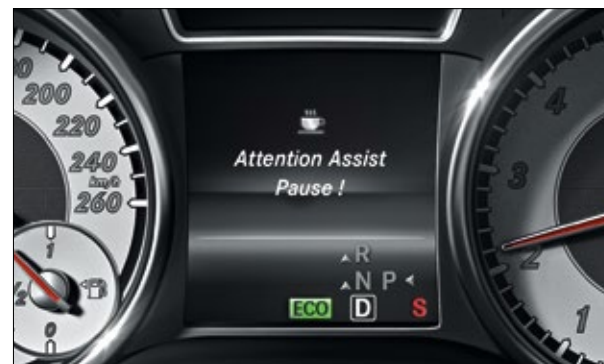
Attention Assist recommends taking a break if the system detects signs of tiredness or inattentiveness
