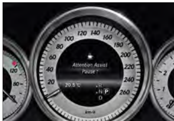
If it detects signs of fatigue or concentration lapses, Attention Assist suggests taking a break
