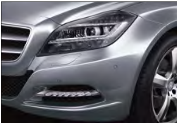
High-performance LED headlamps with LED daytime running lights 2
