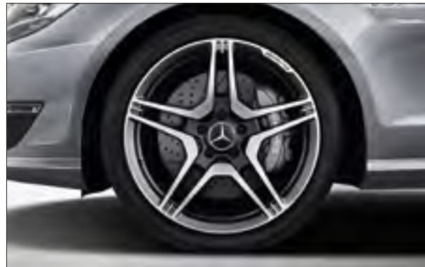
19" AMG 5-twin-spoke forged alloy wheels with polished Titanium Grey finish (optional on CLS 63 AMG, code 793)
