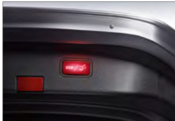
Easy-pack automatic powered tailgate (Shooting Brake only)
