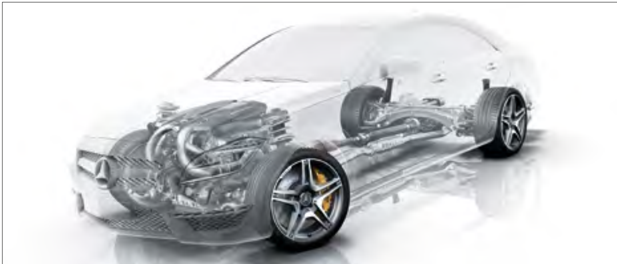
The AMG sports suspension with Ride Control offers variable settings
