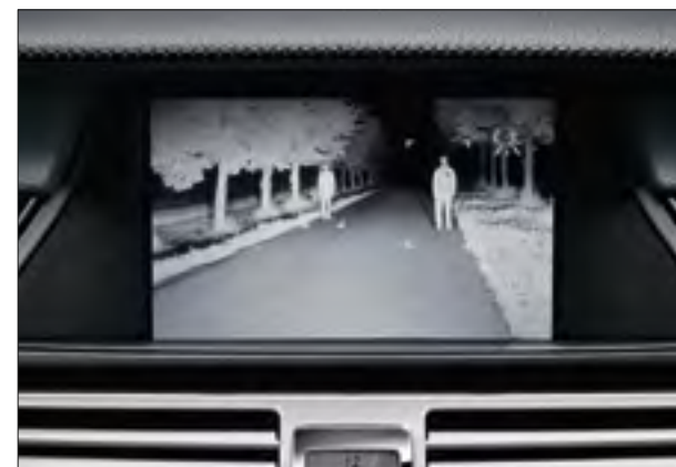
Night View Assist helps drivers to spot pedestrians by highlighting them on the screen
