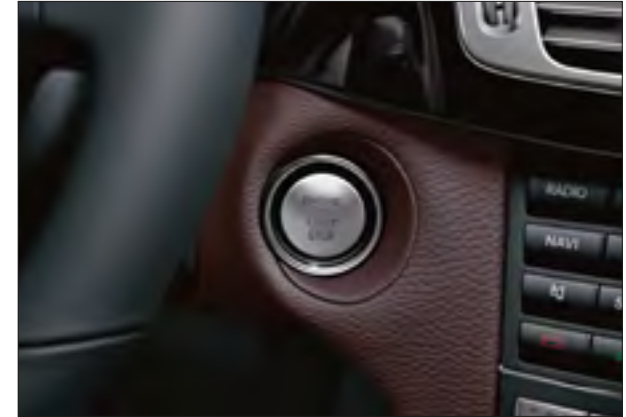
Keyless-Go (including start/stop button)
