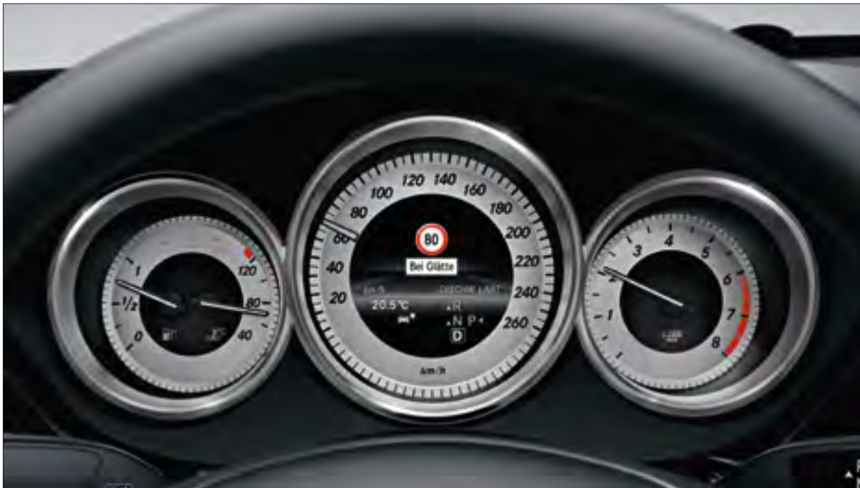
Speed Limit Assist recognises and displays temporary speed restrictions
