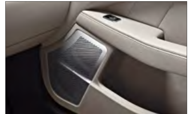
Concert-hall feeling: 14 or 15 speakers are combined with a 1,200-watt DSP amplifier in the Bang & Olufsen BeoSound high-end surround sound system
