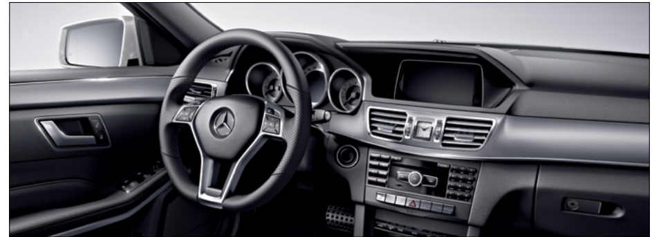
Nappa leather-clad AMG 3-spoke steering wheel with flattened bottom section
