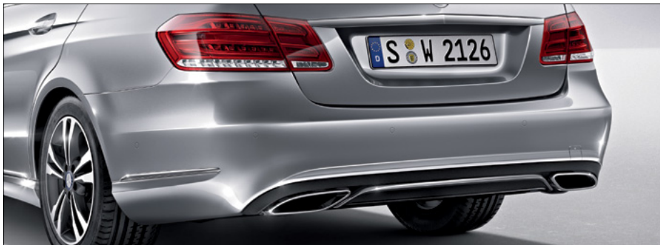
LED rear tail lights and twin-pipe exhaust system with squared, integrated tailpipes in stainless steel are standard
