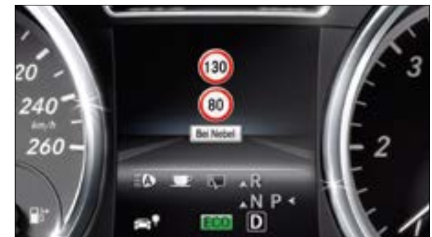
Speed Limit Assist shows you the current legal limit on the instrument panel and in COMAND Online's central display
