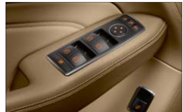
Controls for the electrically-adjustable mirrors
