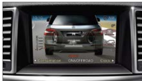
The COMAND Online display shows the current driving mode along with the gradient and angle of inclination
