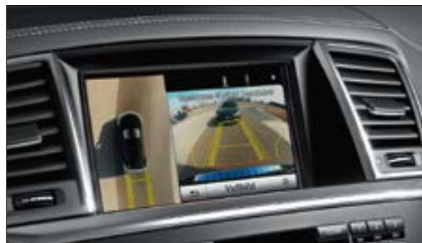
The 360° camera provides a bird's-eye view of the vehicle's immediate vicinity
