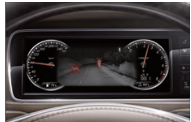
Night View Assist Plus displays detected pedestrians and helps the driver to react sooner to any potential danger
