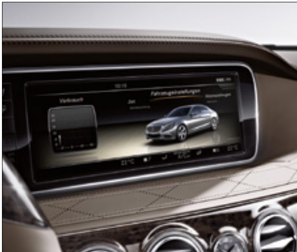
SplitView enables the COMAND Online screen to display different images for the driver and the front seat passenger
