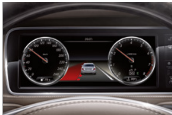
Active Lane-Keeping Assist helps steer the S-Class back on its path when accidentally leaving lane
