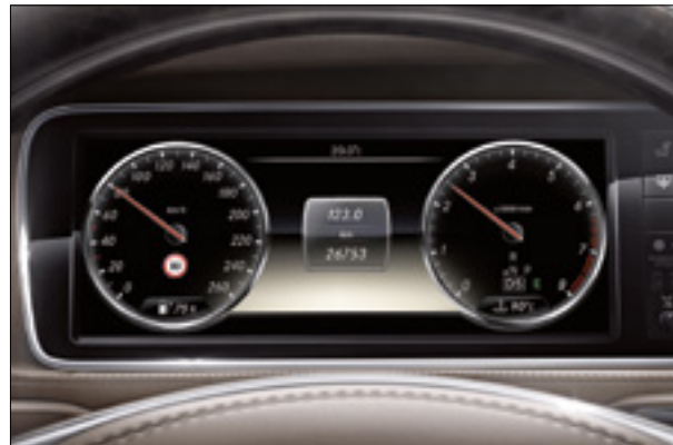
Traffic Sign Assist can detect speed limits and displays the permitted maximum speed in the COMAND display
