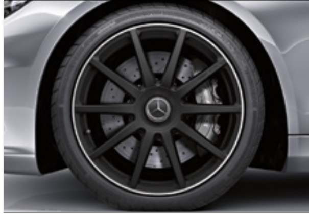
20" AMG 10-spoke forged wheels, matt black lacquer and burnished rims, with 255/40 R20 front and 285/35 R20 rear tyres (S 63 AMG L only, code 648)
