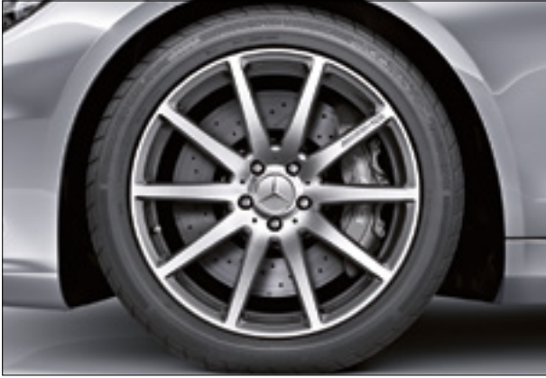
19" AMG multi-spoke forged wheels, polished Titanium Grey finish, with 255/45 R19 front and 285/40 R19 rear tyres (standard on S 63 AMG L, code 788)
