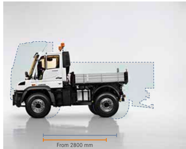
Short wheelbase, compact dimensions: The Unimog implement carrier is extremely agile
