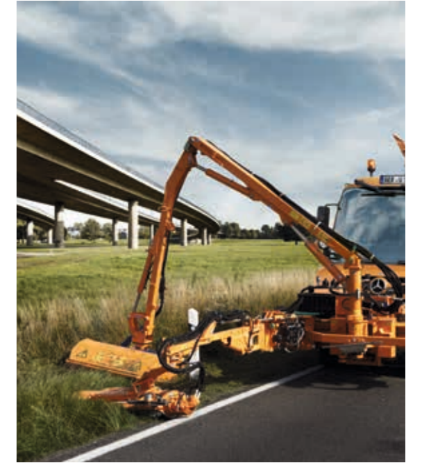
With its hydraulic systems, the Unimog is able to do up to three jobs at the same time with its triple mowing combination
