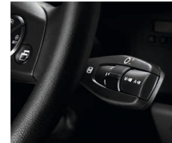
The transmission can be operated easily with the steering column control arm on the right. The premium engine brake is also operated here
