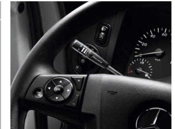
New steering column control arm: Operators can change the driving direction and gear and set the cruise control with their left hand – and have the right hand free to use the multifunction joystick for, e.g. positioning implements
