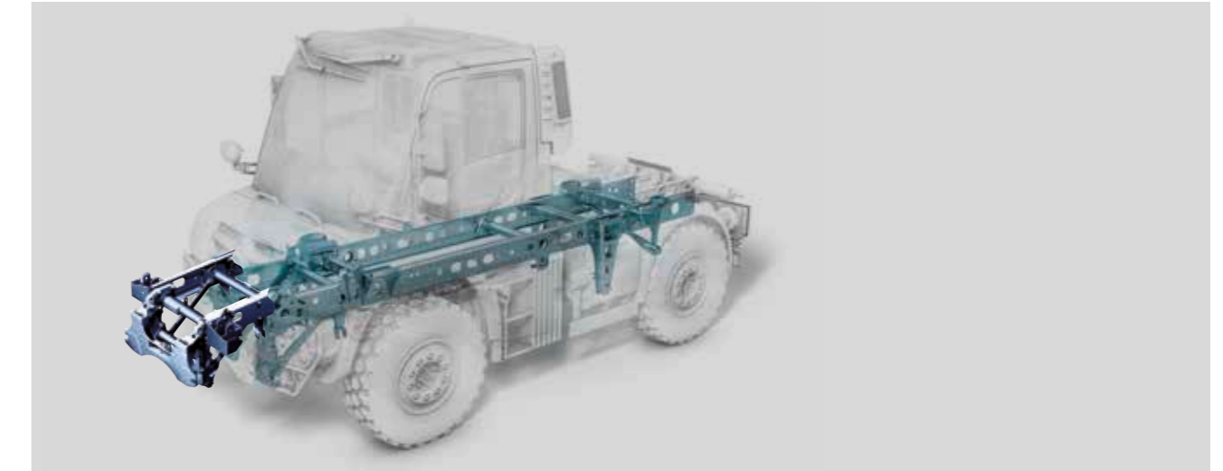
Four attachment and mounting areas: the Unimog implement carrier is one of the most productive working machines in existence. A very wide range of implements can be combined thanks to its standardised interfaces and over 1000 different uses are possible. The system includes the front mounting plate, attachment points on the frame, mounting brackets on the sides and at the rear as well as ball-point positions on the platform sub-frame
