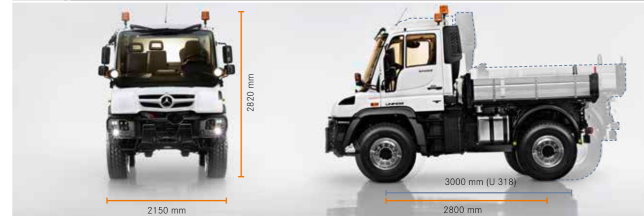
Unimog U 216 and U 218: Technology upgrade for the smallest Unimog. The shorter wheelbases are responsible for the great agility of the vehicles
