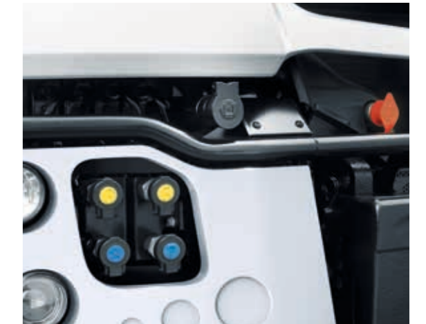
Hydraulic connections for up to four circuits are safely installed at the front and rear of the vehicle
