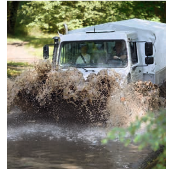
Watertight: High ground clearance, vertical air-intake pipe and protected equipment are suitable for fording depths of up to 800 mm (optional 1200 mm)
