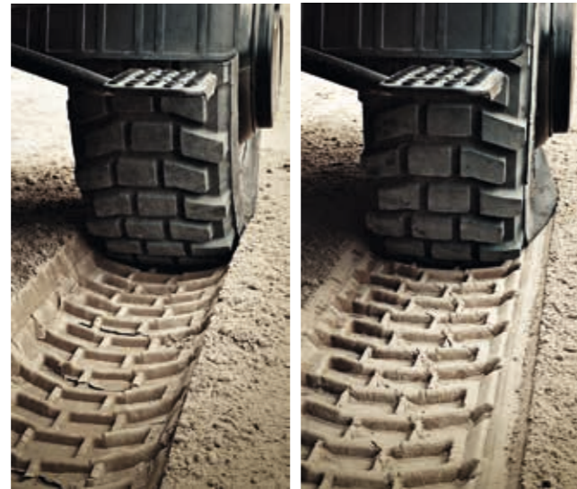
The single-tyre principle: The rear wheels follow in the compacted tracks of the front wheels. This increases traction and is better for the ground surface
