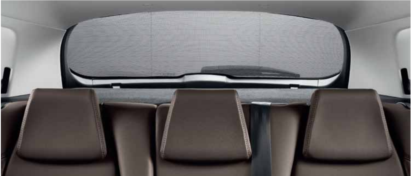
Rear screen sun blind Retractable sun blind for added safety whilst driving in bright driving conditions.
