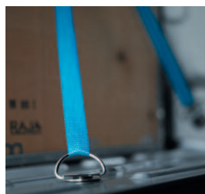
Tie-down hooks The floor has 8 to 10 tie-down hooks according to version (straps not included).
