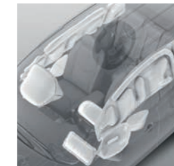
Supplemental Restraint System (SRS) airbags GT86 is fitted with seven airbags including driver's knee airbag.
