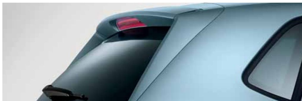
The rear roof spoiler not only enhances the BlueMotion's dynamic lines but also helps to reduce the vehicle's air resistance, and in turn reduces fuel consumption.
