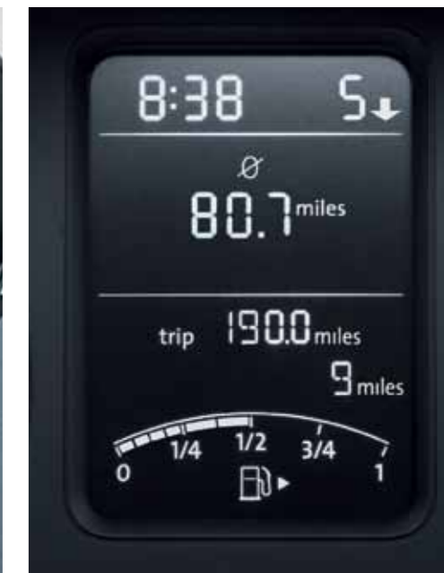
The multifunction computer provides useful statistics about your journey, such as exterior temperature, average and current fuel consumption, average speed and estimated distance to refuelling. It also includes a visual gear change recommendation for improved fuel consumption.
