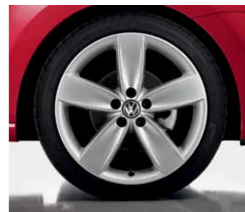
'Boavista' 7J x 17 alloy wheels with 215/40 R17 tyres are eye-catching and stylish, and are fitted with anti-theft wheel bolts. Optional on SEL models.
