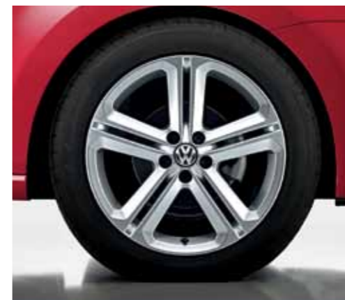
'Mallory' 7J x 16 alloy wheels with 215/45 R16 tyres and anti-theft wheel bolts emphasise the sporty appeal of the Polo R-Line. Standard on R-Line models.
