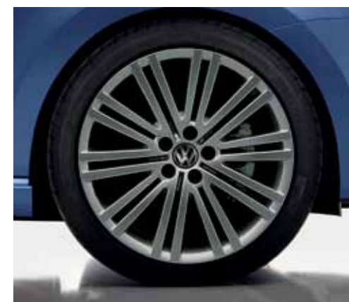
'Montani Anthracite' 7J x 17 alloy wheels with 215/40 R17 low rolling resistance tyres and anti-theft wheel bolts offer an alternative look to the Polo BlueGT. Available as a no cost option on BlueGT models.
