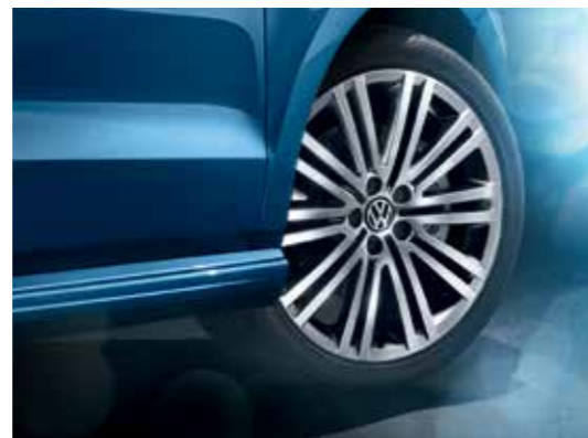
'Montani' 7J x 17 inch alloy wheels with 215/40 R17 tyres are a real design feature of the BlueGT, leaving a lasting impression.
