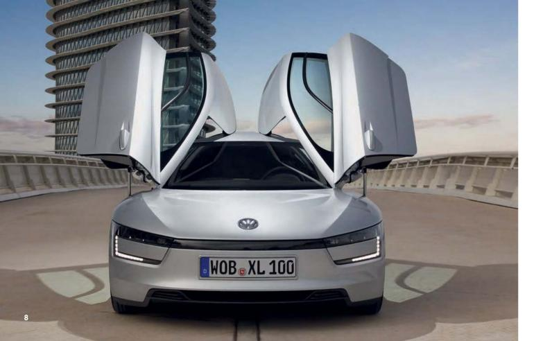
**Wolfsburg, February/March 2013.** The XL1 from Volkswagen is the most fuel-efficient production car in the world, with a fuel consumption value of 0.9 I/100 km. Thanks to its plug-in hybrid system, the two-seater can also cover a distance of up to 50 km in all-electric mode and therefore with zero local emissions.
