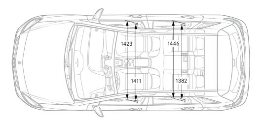
All dimensions in millimetres. The dimensions shown are mean values and apply to standard-specification, unladen vehicles. The dimensions shown correspond to vehicles with a diesel or petrol engine. For the B 200 Natural Gas Drive some of these data can vary.
