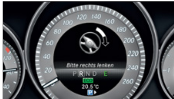
Parking Guidance helps the driver choose the correct steering angle and turn-in point
