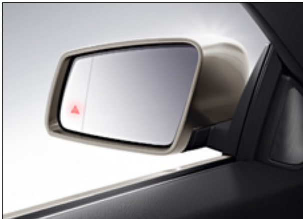
Lane-Keeping Assist and Blind Spot Assist can alert the driver in potentially dangerous situations; for example, when changing lanes
