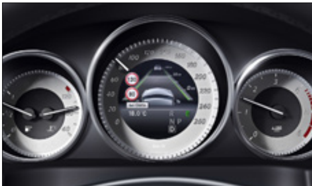
Traffic Sign Assist shows the driver what speed limits and traffic signs apply
