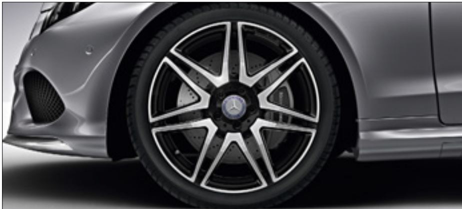
19" AMG 7-twin-spoke bi-colour alloy wheels with front 235/35 R 19 and rear 255/30 R 19 tyres (standard on E 400 AMG Sport Plus or as part of the AMG Sport Plus Package, code 662)
