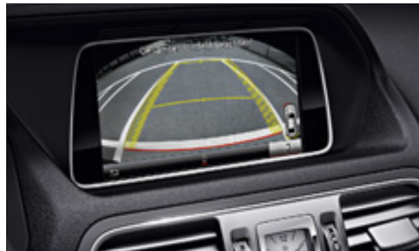
The optional reversing camera supports static and dynamic guides in reversing operations
