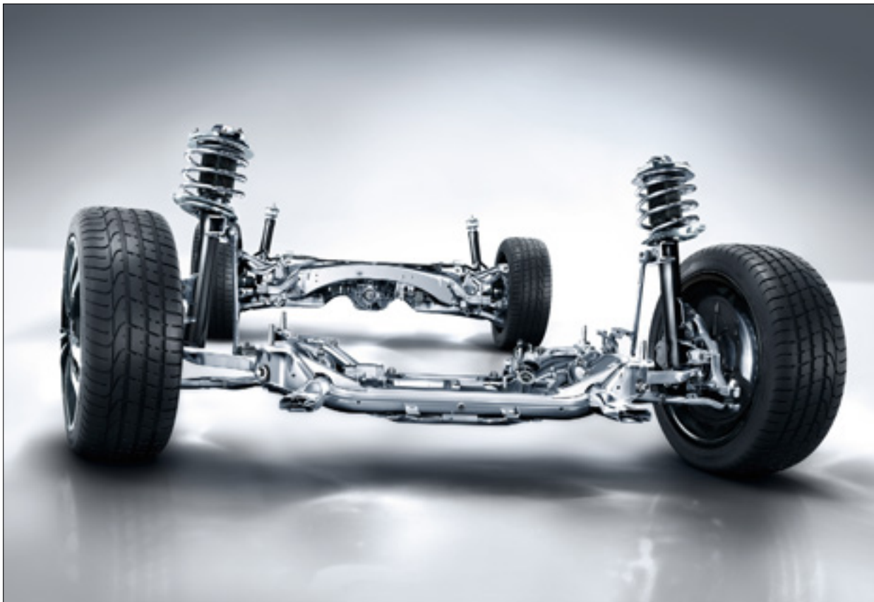
The Agility Control suspension with Adaptive Damping System adjusts to the road conditions offering both agility and comfort on all surfaces
