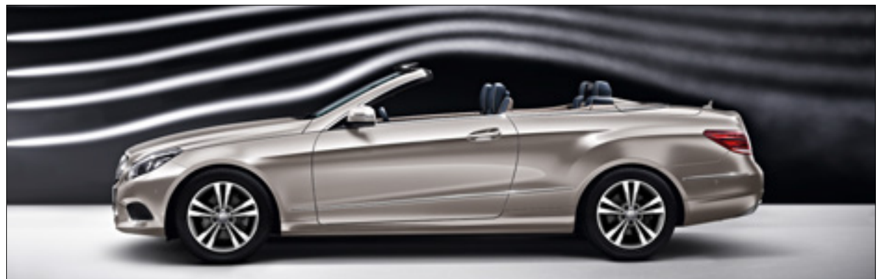
Simply smart: Aircap forces the airflow upwards, above the four passengers' heads
