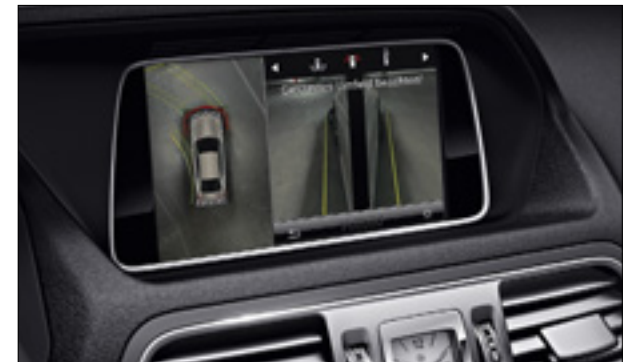
The central display of the COMAND Online system shows the area around the vehicle during parking
