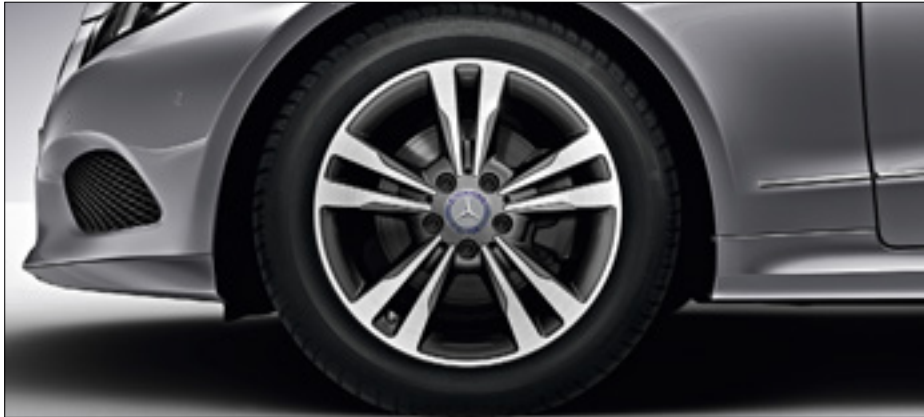
17" 5-twin-spoke alloy wheels with 235/45 R 17 tyres (standard on SE, code 44R)
