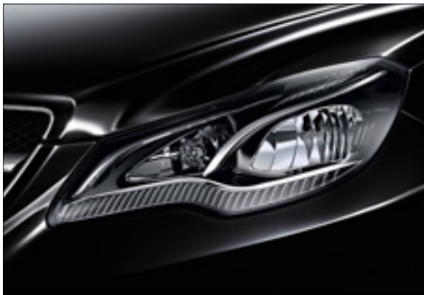
Partial LED headlamps – indicators and high beam are halogen
