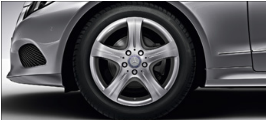
17" 5-spoke alloy wheels with front 235/45 R 17 and rear 255/40 R 17 tyres (optional on SE, code R22)
