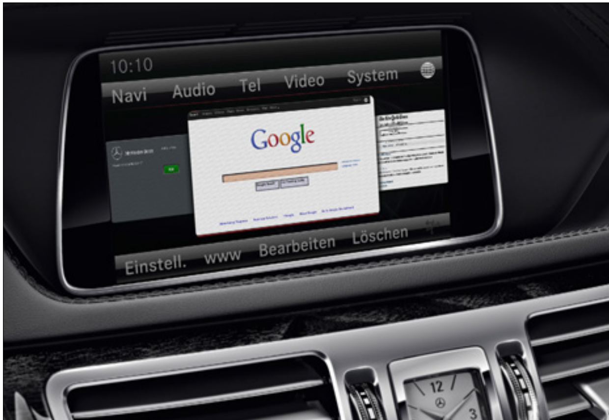
COMAND Online combines audio system, navigation system and telephone functions. All of the main settings can be programmed using Linguatronic voice control
