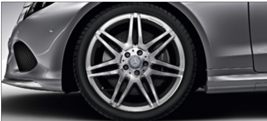
19" AMG 7-twin-spoke alloy wheels, with front 235/35 R 19 and rear 255/30 R 19 (optional on AMG Sport, code 770)
