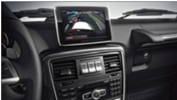
The reversing camera uses the central display to show you what's immediately behind the car
