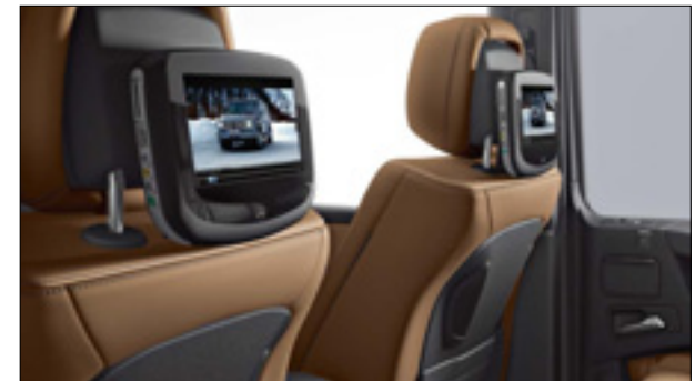
The rear seat entertainment system's twin displays are attached to the backs of the front seat head restraints
