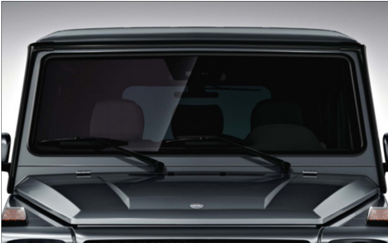
The heated windscreen can be activated at the touch of a button
