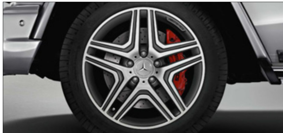
20" AMG 5-twin-spoke alloy wheels with burnished Titanium Grey high sheen finish and 275/50 R 20 tyres (standard on G 63 AMG 4MATIC, code R10)
