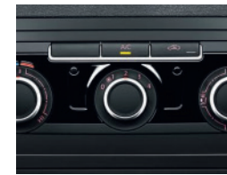
Climatic manual air conditioning.
