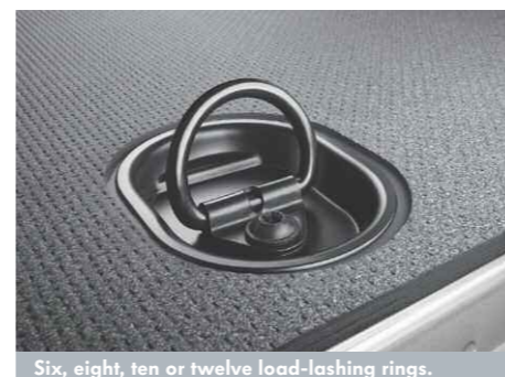
Six, eight, ten or twelve load-lashing rings.
