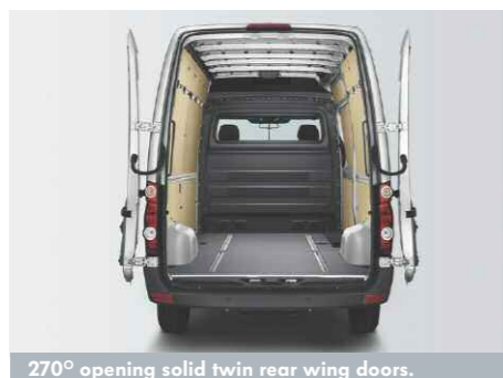
270° opening solid twin rear wing doors.
