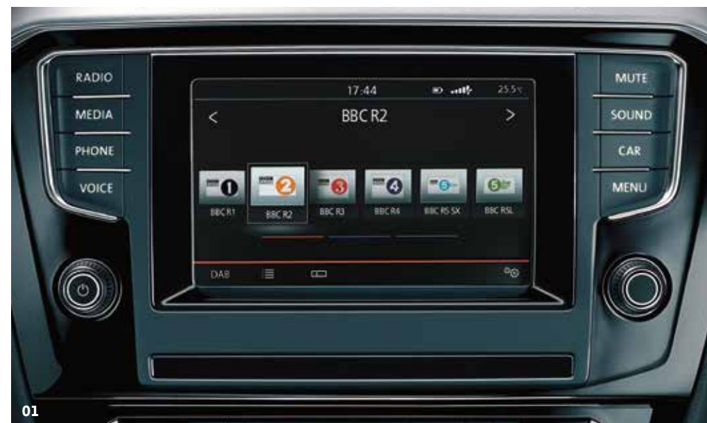
01 The Composition Media system is equipped with a 6.5 inch colour touch-screen with proximity sensor that recognises in advance your intention to touch the screen and automatically magnifies the display mode. Features also include DAB digital radio receiver, CD player, MDI (Multi Device Interface) via USB connection, SD card reader and SMS functionality – allowing you to read, compose and send SMS messages using the touch-screen display (compatible Android smartphones only). It also features title and compatible cover art display and facilitates music playback from MP3, WMA and AAC files through eight speakers front and rear with 4 x 20 watt output. Car information display and Think Blue. Trainer. – provide journey analysis and driver tips for more fuel efficient driving. Standard on S and SE models.
