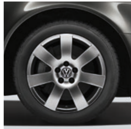
'Innovation' 8½J x 18 inch alloy wheels with 255/45 R18 tyres and anti-theft wheel bolts. Available as a no cost option on the LWB model.
