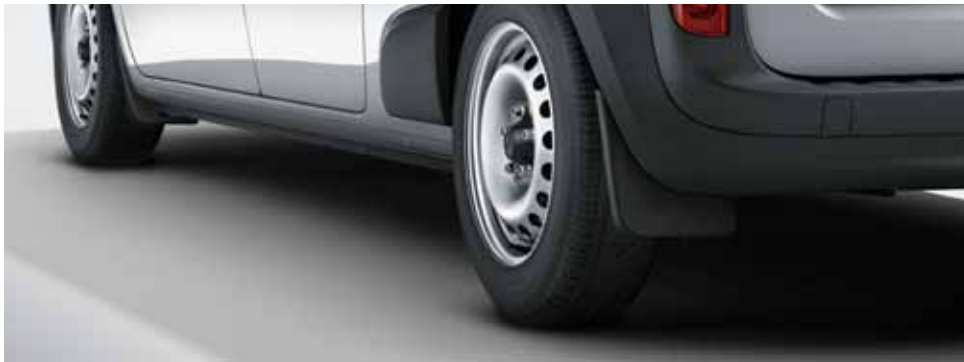
Mud flaps. These flaps protect against dirt and scratching in the area of the side walls, rear end and underfloor.
