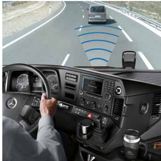
Proximity Control Assist 1) . The safety system with stop-and-go function is on hand to support the driver in stressful situations and reduces the risk of rear-end collisions.
