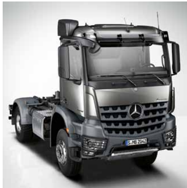
ClassicSpace S-cab. The 2300 mm wide and 1700 long cab with an engine tunnel height of 170 mm or 320 mm is tailored to the requirements of one-man operations in construction transport and offers excellent visibility.
