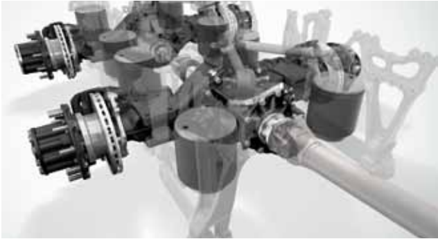
Rear axle, crown wheel 440, hypoid, 13.0 t. The rear axle is a weight-optimised sheet-steel formed axle with a 440 mm ring gear. It is fitted to air-suspended 3-axle vehicles up to a gross train weight of 80 t.
