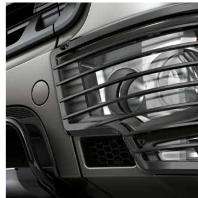
Protective headlamp grille. Robust protective steel grilles are available for the headlamps and tail lamps of the Arocs. They can prevent damage such as stone chips, for example. This contributes to low repair costs and enhanced safety.
