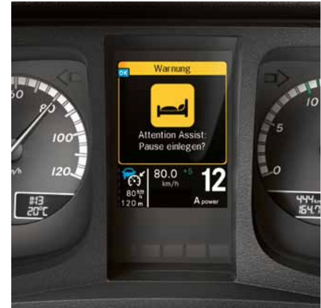
Attention Assist 2) . The system can recognise increasing tiredness and recommend the driver takes a break.
