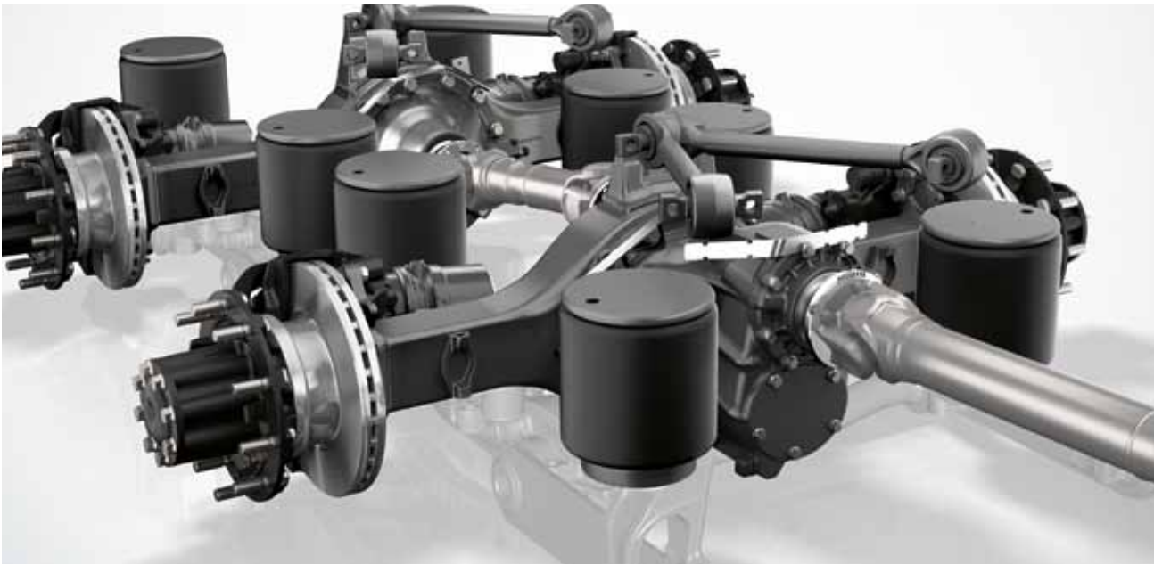
Rear axle, crown wheel 390, hypoid, 10.0 t. The rear axle is a weight-optimised sheet-steel formed axle with a 390 mm ring gear. It is fitted to air-suspended 3 and 4-axle vehicles up to a gross train weight of 44 t. It has a single ratio. The hypoid toothing ensures high running smoothness with low frictional losses. The drive shafts have maintenance-free compact bearings; the wheel bearings are also maintenance-free.
