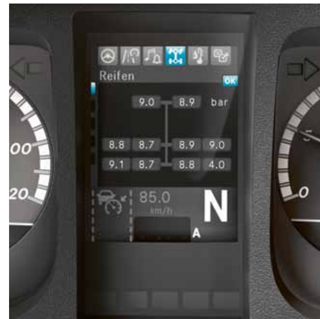
Tyre pressure monitoring 2) 4) . The wireless pressure monitoring system for the front and rear axles continuously monitors the air pressure in all the tyres of the tractor unit as well as those of the semitrailer or trailer.
