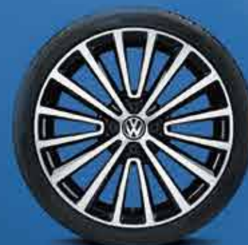
'Polygon' alloy wheels† 6½J x 17", 195/40 R17 tyres | High up! Street up! includes sports suspension
