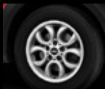
5-Hole Circular Spoke R123 light-alloy wheel in Silver Size 6.5J×16 1
