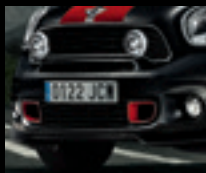
Front apron featuring aerodynamic splitter
