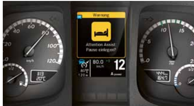
Attention Assist 7) 9) . The system can recognise increasing tiredness and recommend the driver takes a break.
