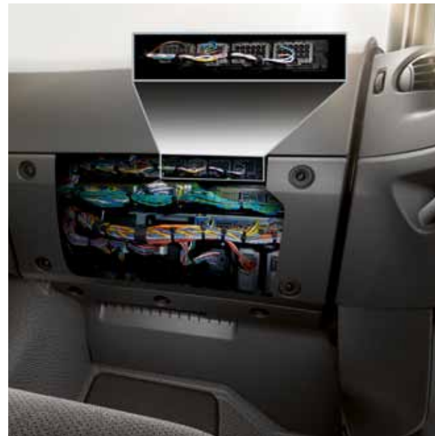
Parameterizable special module 1) . The parameterizable special module (PSM) provides for perfect information processing and a smooth exchange of information between vehicle and body.
