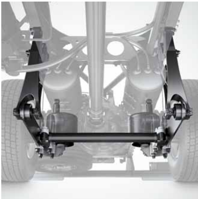
Stabiliser, rear axle. The robust stabiliser reduces vehicle roll and thus offers greater safety and comfort. It is situated under the frame at the rear axle.
