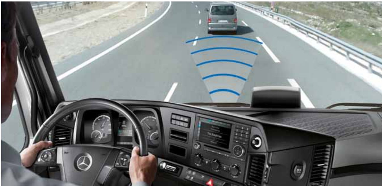
Proximity Control Assist 1) 2) . The safety system with stop-and-go function is on hand to support the driver in stressful situations and can reduce the risk of rear-end collisions. When approaching an identified vehicle driving ahead, the system reduces the speed and maintains the preset distance.
