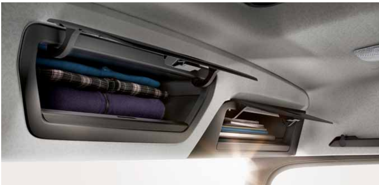
Storage flaps above windscreen. The flaps prevent objects from falling out of the stowage compartments and protect the contents from prying eyes.
