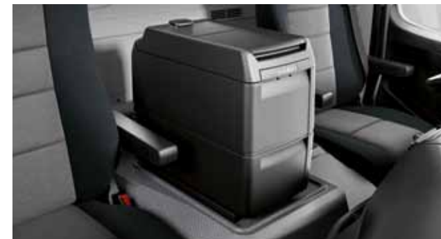
Coolbox on engine tunnel 1) . Bottles and food can be stored separately in the coolbox fitted on the engine tunnel. The lid also serves as a document holder and as a step for accessing the top bunk.
