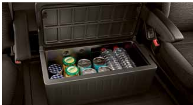
Refrigerator on engine tunnel 2 . The coolbox provides the driver with cold drinks and food. It can be reached easily from the driver's seat and makes the driver less dependent on service areas.
