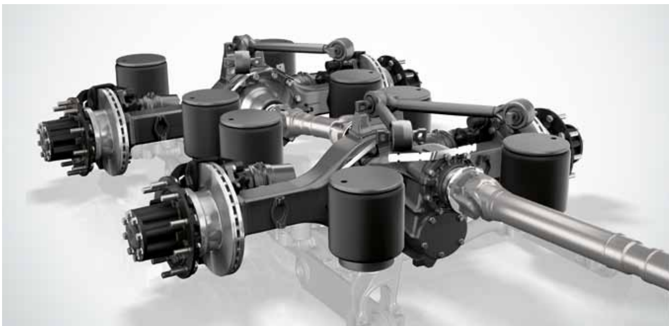
Rear axle, crown wheel 390, hypoid, 10.0 t. The rear axle is a weight-optimised sheet-steel formed axle with a 390 mm ring gear. It is fitted to air-suspended 3- and 4-axle vehicles up to a gross train weight of 44 t and up to 2100 Nm. It has a single ratio. The hypoid toothing ensures high running smoothness with low frictional losses. The drive shafts have maintenance-free compact bearings; the wheel bearings are also maintenance-free.
