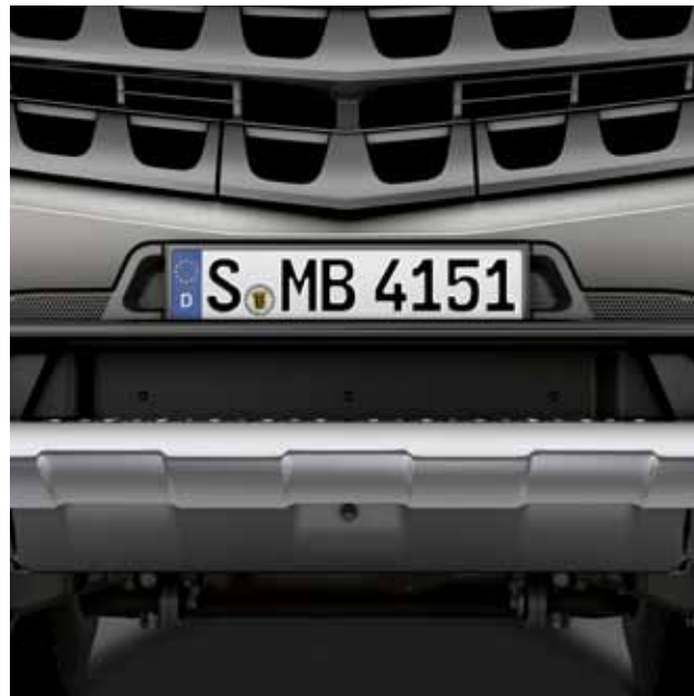
Protective plate for engine and radiator. Many off-road models come with a steel plate to protect the radiator and the engine. A strong protective plate for the main tank is also available as an optional extra.
