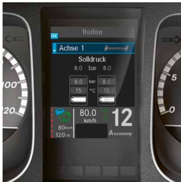
Tyre pressure monitoring 2) 4) . Wireless pressure monitoring permanently monitors the tyre pressure and shows the specified pressure required for the tyre temperature on the basis of the outside temperature.
