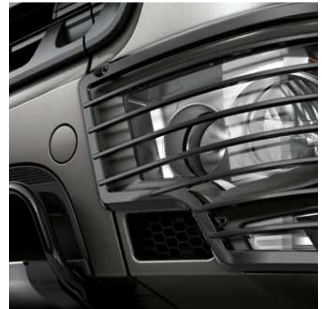
Protective headlamp grille Robust protective steel grilles are available for the headlamps and tail lamps of the Arocs. They can prevent damage as caused by stone chips, for example. This contributes to low repair costs and enhanced safety.
