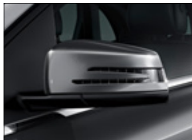
Automatically dimming driver's exterior mirror
