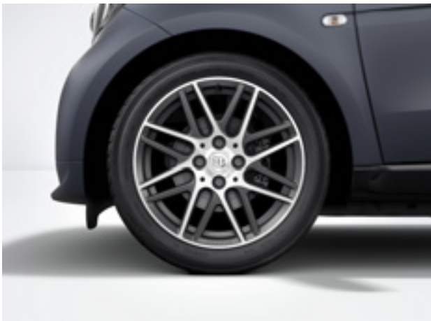
16/17-inch BRABUS Monoblock IX alloy wheels (R80) painted in matt grey with a high-sheen finish, with front tyres 185/50 R16, rear tyres 205/40 R17
