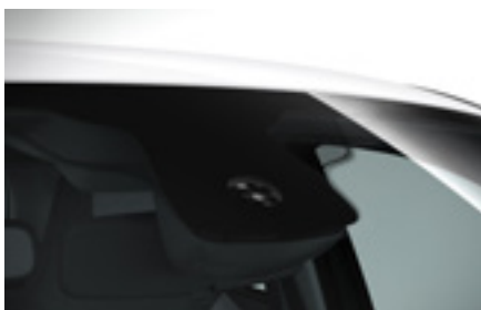
Rain/light sensor: rain sensor controls the windscreen wipers, adapting wipe intervals to amount of rainfall. The accompanying light sensor automatically activates driving lights
