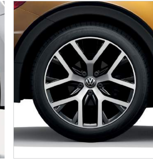
18 inch 'Mythos' alloy wheels with 235/45 R18 tyres and anti-theft wheel bolts are standard on Dune models. Image shown features optional Sandstorm Yellow metallic paint.
