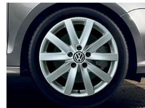
'Porto' 7J x 17" alloy wheels with 225/45 R17 tyres and anti-theft wheel bolts. Optional on SE and GT models. SE models include sports suspension lowered by approx. 15mm.
