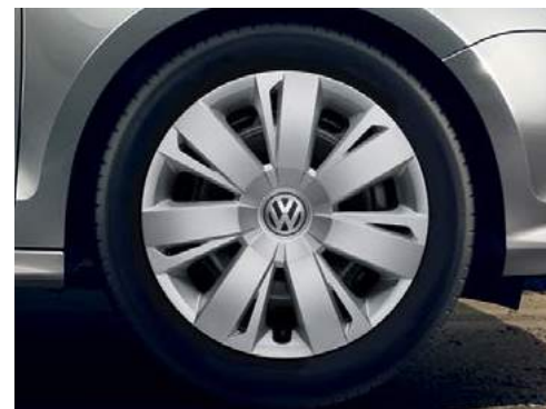
6½J x 16" steel wheels with 205/55 R16 low rolling resistance tyres and full size wheel trims. Standard on S models.
