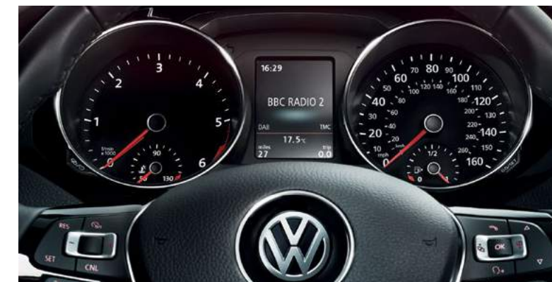
The large 3.5" TFT colour screen of the multifunction computer displays important driving information such as journey time, outside temperature, range left in the fuel tank, total driving time and the status of your connected mobile phone. Standard on GT and optional on SE models.
